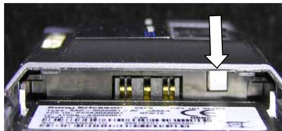
Location of the Liquid Intrusion Indicator. (Remove battery cover and battery)
